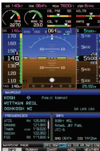
Single screen with engine instruments, PFD and destination information page or other MFD-like information
